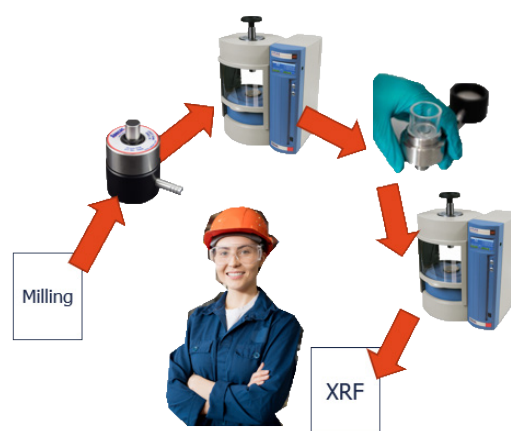
Schematic of the workflow for pressing with manual dies
